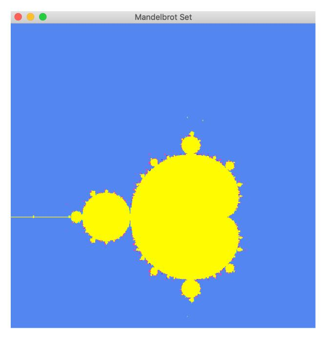
This Python program graphs the Mandelbrot set using an array of pixels that correspond to the divergence of  $f(z)=z^2+($ the complex number x+yi at (x,y))
